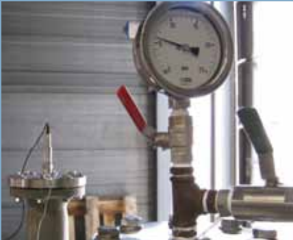
Hydrostatic test of a vessel with PED approval
