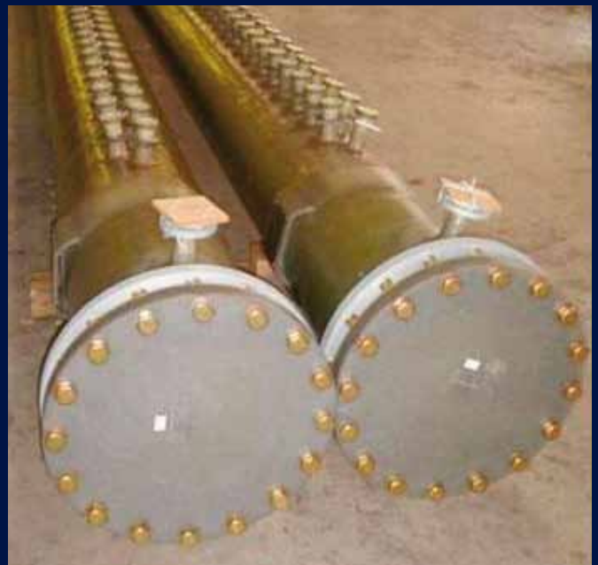
Two catholyte PP, GRP headers for the chlorine industry
