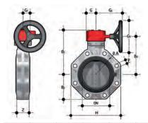
**FKOF/RM LUG ISO-DIN**Gearbox operated Butterfly valve, version Lug ISO-DIN
