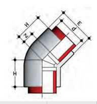
**HIF** 45° elbow for socket welding
