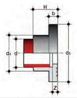
Stub with serrated face for socket welding, for used with backing rings OAB (for other dimensions use QRNF)
