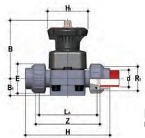
**DKUIF**DIALOCK® diaphragm valve with female union ends for socket welding, metric series
