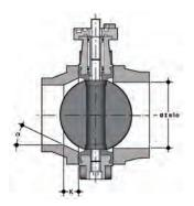
Before proceeding with the installation of the stubs, check that the bore of the fittings has sufficient clearance to allow the valve disk to open correctly.
