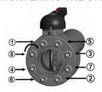
Before tightening the stud-bolts, it is advisable to open the disk in order to prevent damage to the seal. Tighten the stud-bolts in a uniform manner, in the order indicated in the figure, to the nominal operating torque value indicated in the table. The stud-bolts do not need to be excessively tightened in order to produce a perfect hydraulic seal. Overtightening could adversely affect the operating torque of the valve.
