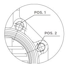
Place the inserts in the holes according to the positions indicated in the table, from the side corresponding to the letters D and DN in order to facilitate the insertion of the stud-bolts and the coupling with the flanges (DN  $40 \div 200$ ). The self-centring inserts must be inserted in the guides in the slots in the valve body on the side with the writing, with the writing facing upwards, and positioned according to the type of flange drilling, as indicated in the following table:
