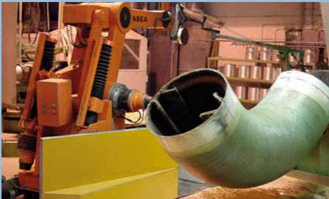
Fully robotized production of a GRP elbow (D < 1200 mm)
