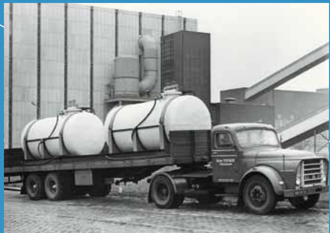
Transport of horizontal PVC/GRP tanks for a chemical plant in the Netherlands in 1959
