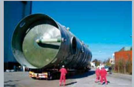
Transport of a GRP scrubber of D = 4 meter for a waste incineration plant in Germany
