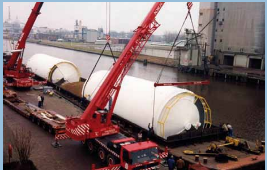
Loading of two tanks of 1000 m 3 for delivery to the Far East by sea transport
