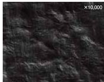
電顕写真 Micro Scope Photograph of the inside surface of PVDF-UHP pipe
